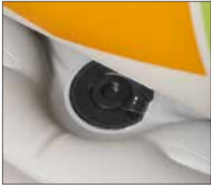
1+2 or 1+4 superfast self-bailing drain valves
