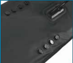
1+8 or 1+16 superfast self-bailing drain valves that can be left open in whitewater and ocean kayaking conditions
