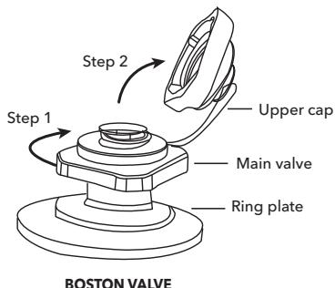
3. Start pumping air into the kayak. Keep inflating until the required air pressure is reached. DO NOT OVERFILL. Once inflated, firmly cap each valve.
