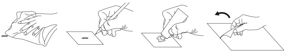
A leaking valve is rare, but if you do find a leak, turn to after-sales service center for a replacement valve. To locate a leak, we recommend mixing soap and water in a spray bottle, spray around the valve. If you see bubbles forming, check your valve seating and base and be sure the valve insert is screwed tight. If the kayak is losing air and all the valves are good, it probably has a small puncture.
