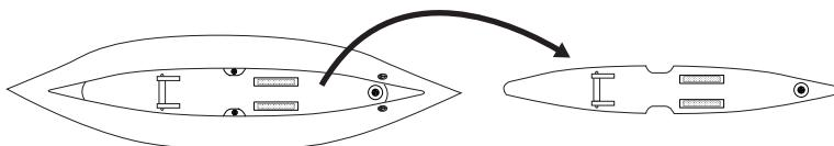
**NOTE:** Remember to remove the DWF air deck floor before folding.
