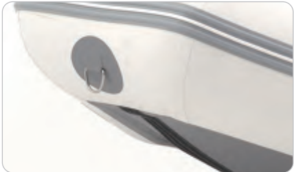
High pressure inflatable keel for excellent water dividing and tracking performance (BT-88810/30 excluded)
