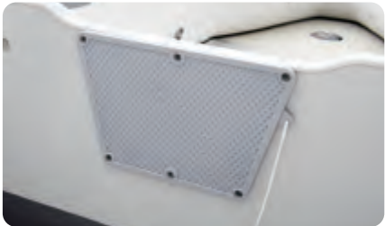
Marine grade plywood transom for outboard motor
