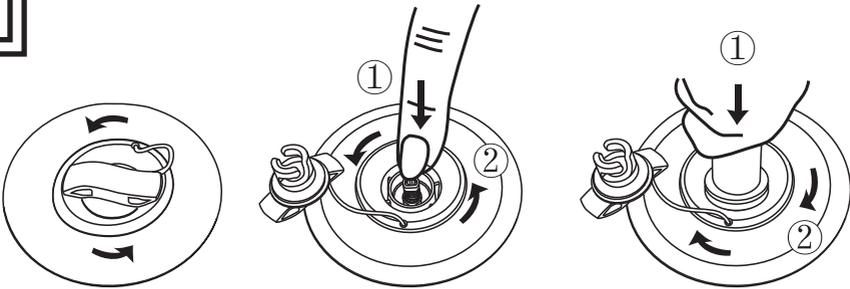
1. Open the valve cap by twisting counter-clockwise. Ensure the valve is clear from debris, sand, or dirt before releasing.
