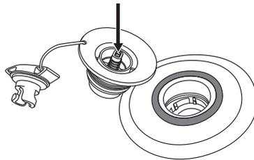
3. Check the rubber ring to make sure that it is in the correct position, tight around the valve and there is no debris in the way.
