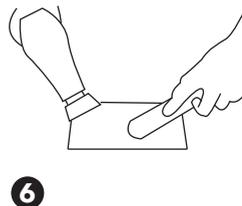
4. Apply glue on both the board and patch using a brush or other applicator. Make sure the glue is spread evenly and completely over the board and patch. Let the glue dry for 5 minutes.
