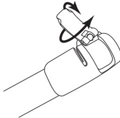
Ensure the center line of the scale is aligned with the indicator on clamp
